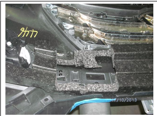
Figure 11: Trim of polystyrene bumper infill
