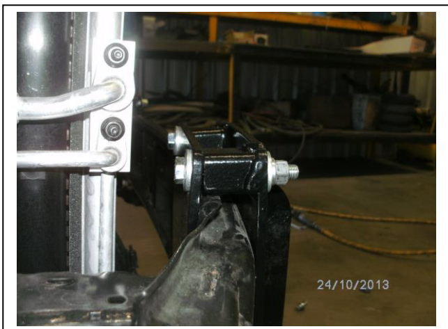
Figure 7: Placement of bolts on mounts
